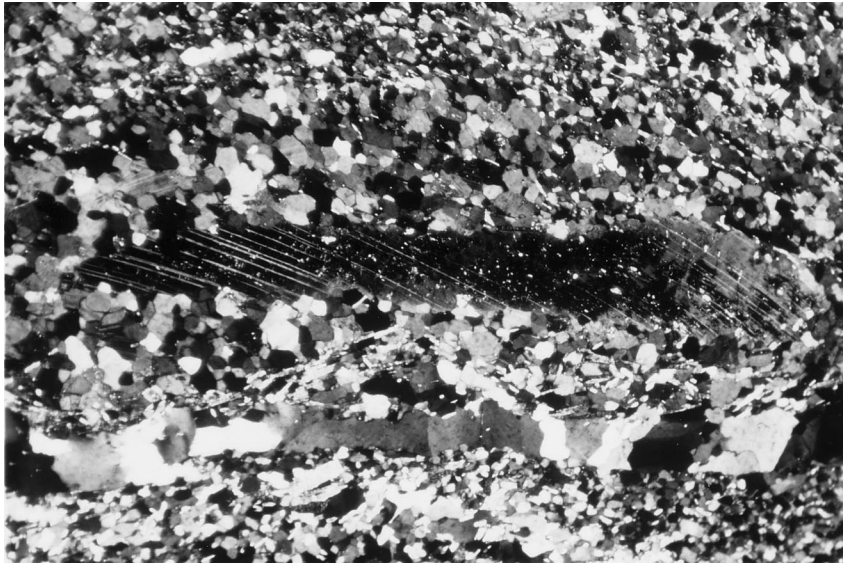
Fig. 14. (010) Twins make a low angle (ca. 10^\circ ) with the long dimension of an elongate plagioclase grain set in a polycrystalline plagioclase mosaic. A well-defined outer limit to the surrounding monomineralic plagioclase mosaic (boundary between monomineralic and polyphase mosaics) indicates the form and volume of the parent grain and demonstrates that the elongate plagioclase is part of a core-and-mantle structure. Long side of photo is 2.8 mm. Crossed polars.
